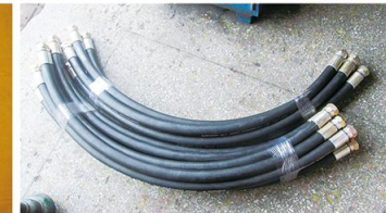
Hydraulic oil pipes
